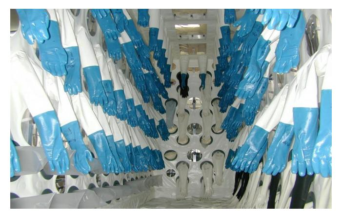
Glove box gloves allow safe handling inside a glove box. Typical applications of these special gloves are:
