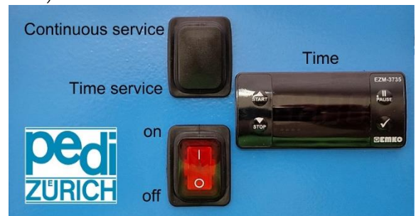
Switches for on/off and operation mode,
