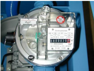
Quantometer of high accuracy. and timer.
