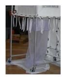
The discharge bag is typically made of soft PVC with a thickness of 0.4 mm. It is translucent and has a built-in O-ring for attachment to a glove port. The design allows contamination-free bag change.
