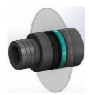
115181 Feed-through inside with connection flange IG M62 (e.g. for HEPA 14 filter, 50 m³/h) outside with hose connection for hose ID = 60 mm
