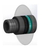
115179 Feed-through inside with connection flange AG ¾" (e.g. for HEPA 14 filter, 5 m³/h) outside with hose connection for hose ID = 60 mm
